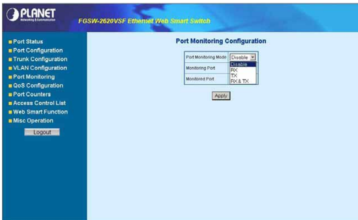
Figure 4-28 Port Monitoring Web Page screen
